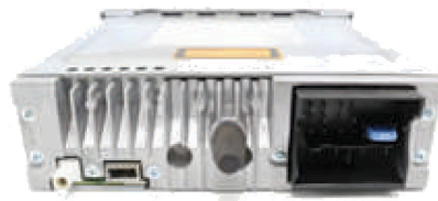
Back of the original radio: look at the shape of the connection.
