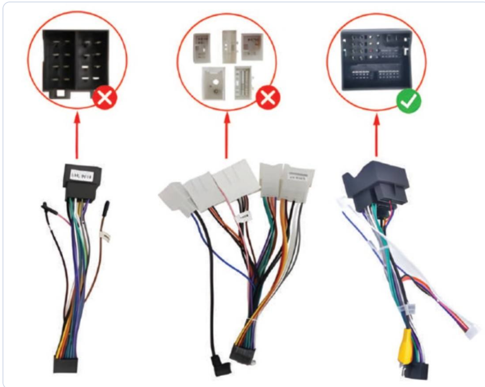
Figure 9-5 Only the cable with the tick fits this car
